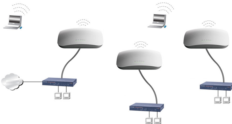
Figure 8. Point-to-multipoint WiFi network
