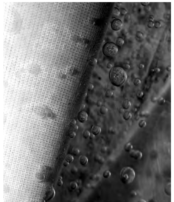
Coalesced water drops releasing from the knitted sock at the outside surface of the cartridge.
