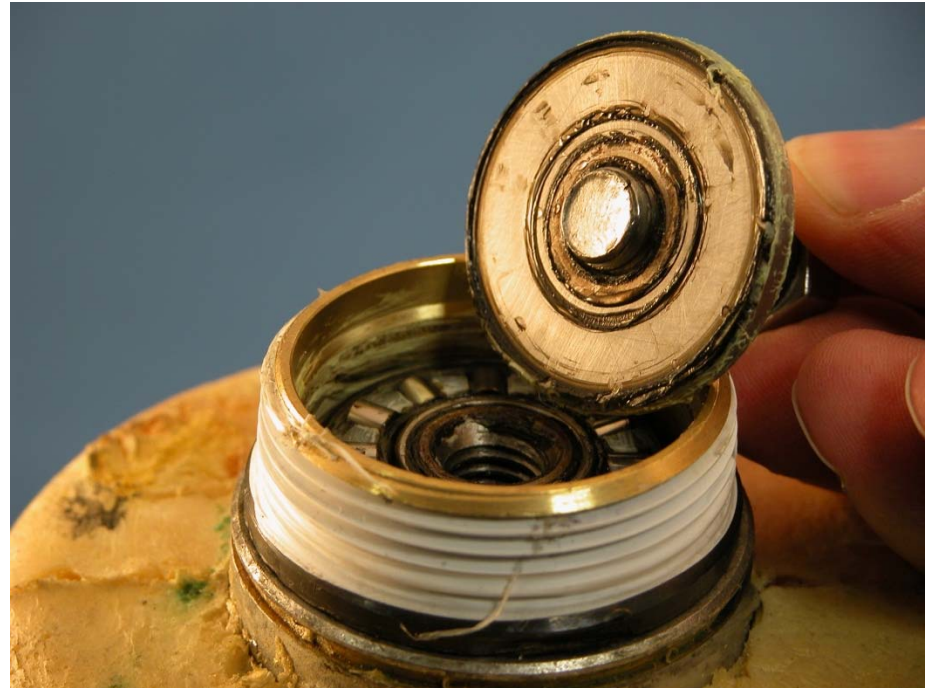
Unscrew Bolt, Remove Thrust Washer
