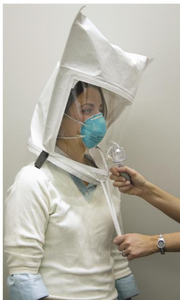
Qualitative fit-test in progress.
