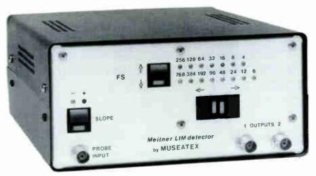
Meitner LIM/Jitter detector/demodulator. The input is connected to the word-clock signal of the device under test; the output consists of an FM-demodulated audio-band signal representing, and proportional in level to the amount of, the time jitter in the word clock.
