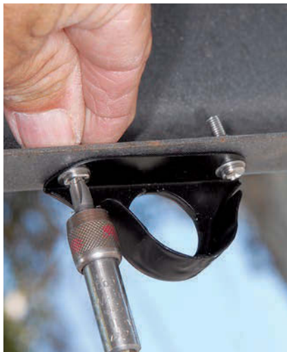
Using the sensor bracket as a template, drill the appropriate holes in the rear bumper. The individual mounting brackets are bolted to the bumper using the provided fasteners.
