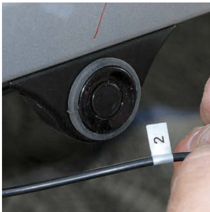
Make sure each sensor is installed in numerical order, beginning at the driver's side.
