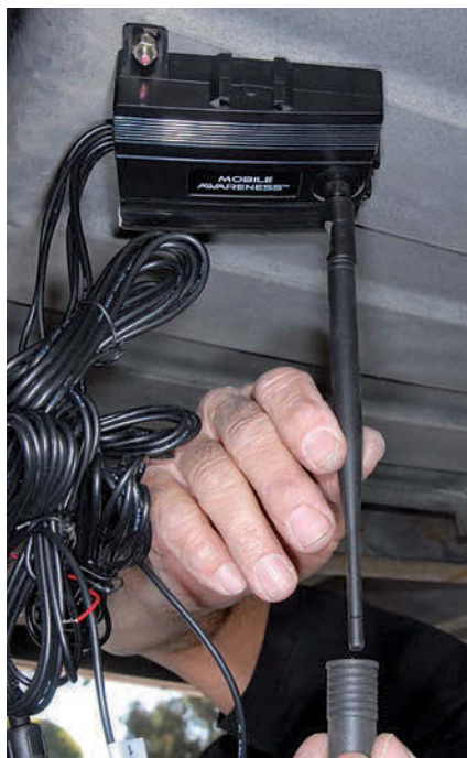
With the ECU bolted in place, install the flexible sleeve over the antenna to prevent it from folding up while driving.
