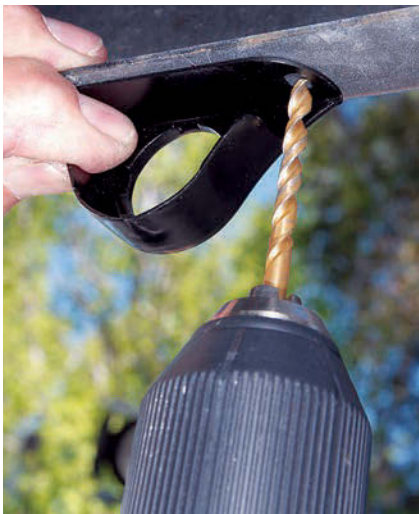
Using the sensor bracket as a template, drill the appropriate holes in the rear bumper. The individual mounting brackets are bolted to the bumper using the provided fasteners.
