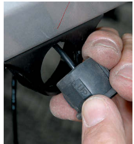
Prior to installing each sensor, be sure that the arrow is facing in the upward position for proper function of the SenseStat.
