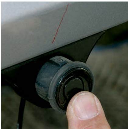
Make sure each sensor is installed in numerical order, beginning at the driver's side.
