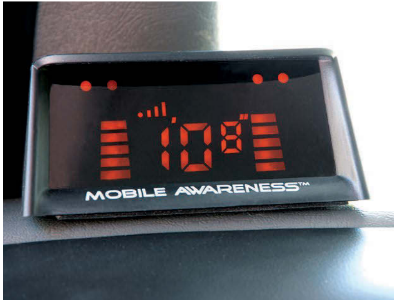
The dash-mounted monitor for the Mobile Awareness SenseStat system offers users a clear readout of specific distances as well as several different audible alert tones.
