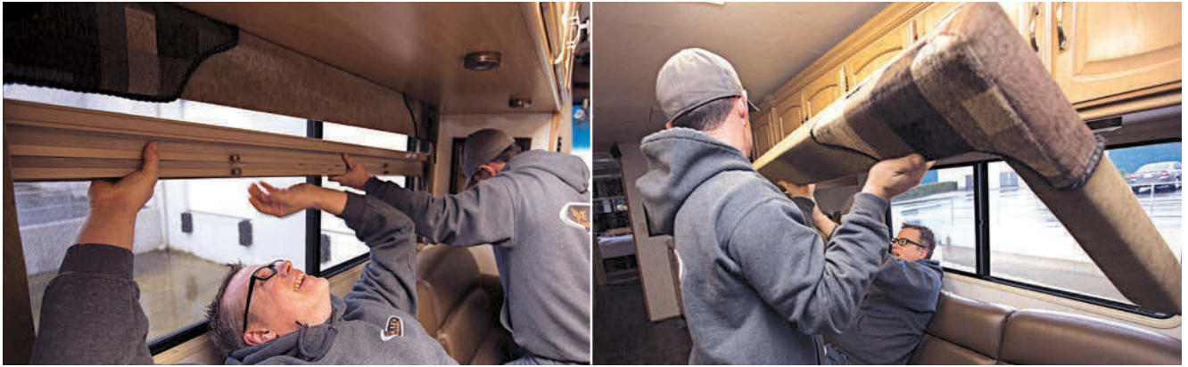
Above left: Old day/night shades are removed before the valance (right) can be unscrewed and pulled from the wall. It may take two people to remove the day/night shades and valances from large windows.
