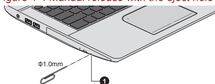
Figure 4-4 Manual release with the eject hole
