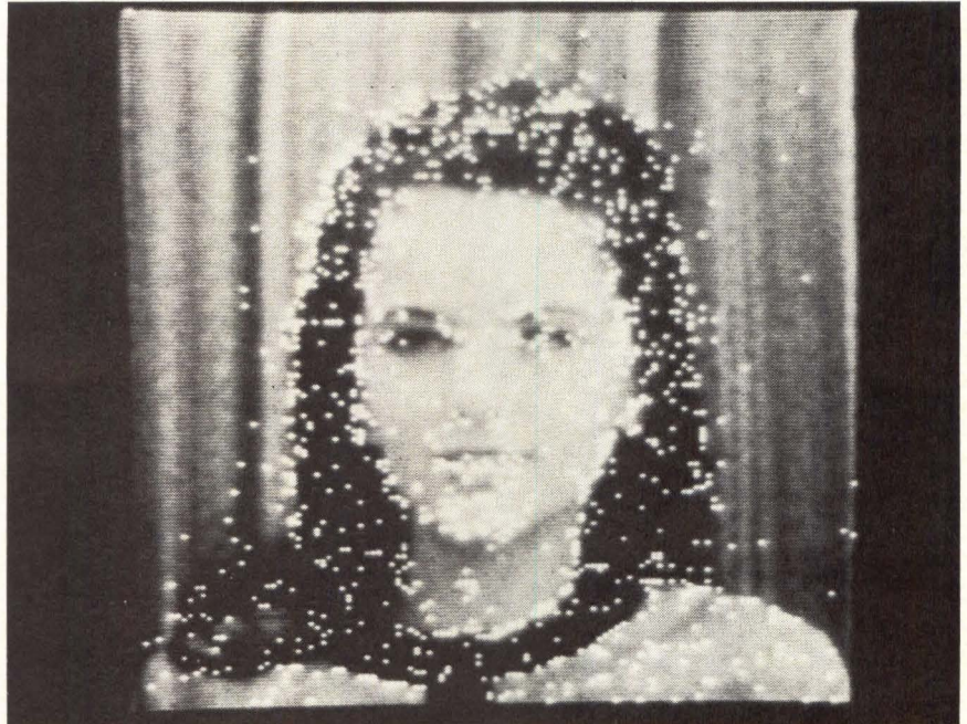
White dots in this actual video-telephone picture show areas of significant change during face-to-face communications in one-sixtieth of a second. An experimental technique (called conditional replenishment) developed by Bell Telephone Labs transmits only these changes to update the previous picture.
