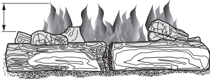
Figure 28 - Correct Burner Flame Pattern
