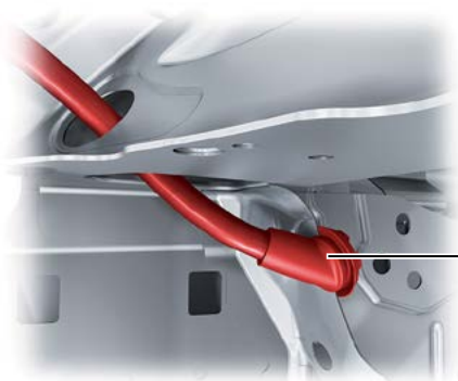
Water drain grommet in plenum chamber
