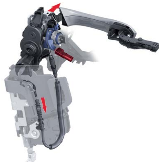
Exterior door operation via a Bowden cable
