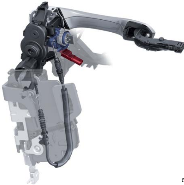
Door handle, support arm and door lock in the rest state.
