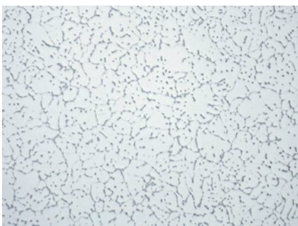
Fig. 3: Aluminium alloy 2024, cast, showing eutectic precipitation on grain boundaries, unetched, 200x.
