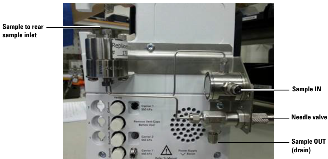
Figure 22 G3581-S0003 pressure regulator assembly installed
