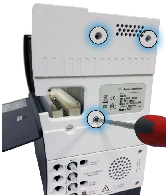
Figure 15 Remove the rear panel by unscrewing the three bolts.
