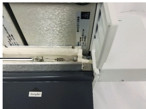
Figure 17 Install the back panel and micro-gasifier, and connect the micro-gasifier sample line to the internal sample inlet using a 1/16-inch Swagelok fitting.
