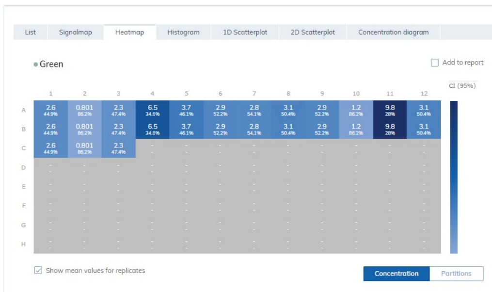
The concentration heatmaps of a selected target (with and without selected mean values for replicates).
