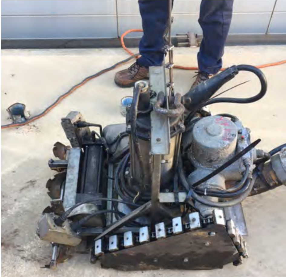
This is the robot used at Toyota's Mississippi assembly plant to clean the cooling tower. Using the robot eliminates the need to drain 80,000 gallons of water during the cleaning process.
