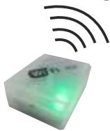
Cm Wifi-box (Internet boiler operation monitoring)
