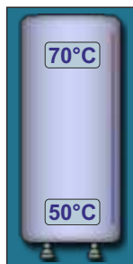
Accumulation tank with current temperature at top of the tank and at the bottom of the tank.
