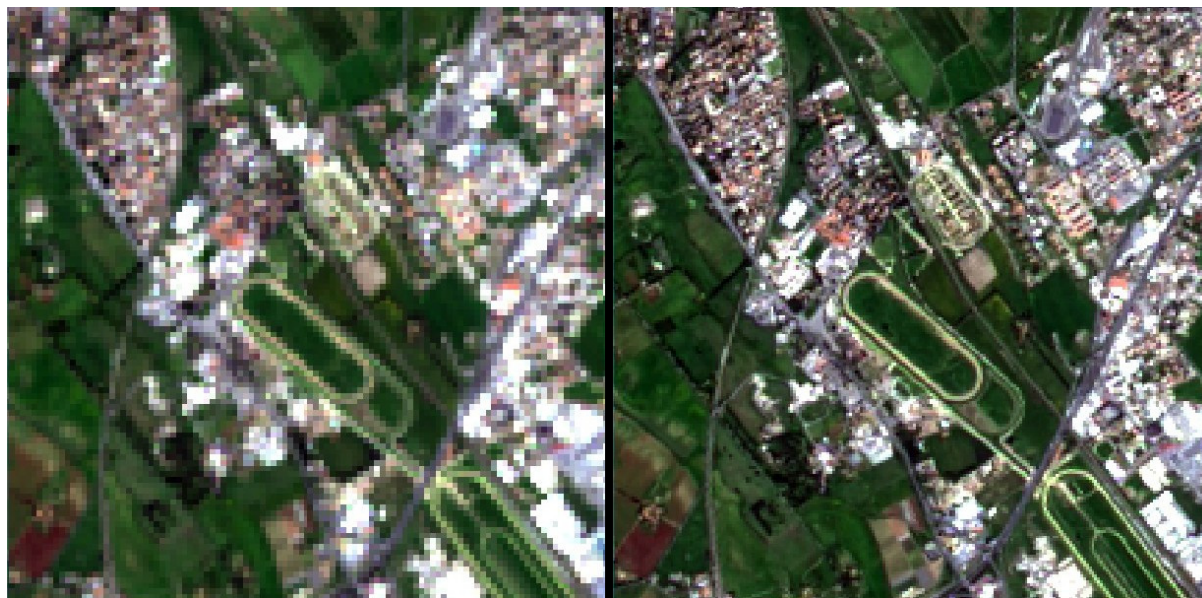
Fig. 14.4: Example of pan-sharpening of a Landsat 8 image. Left, original multispectral bands (30m); right, pan-sharpened bands (15m)
