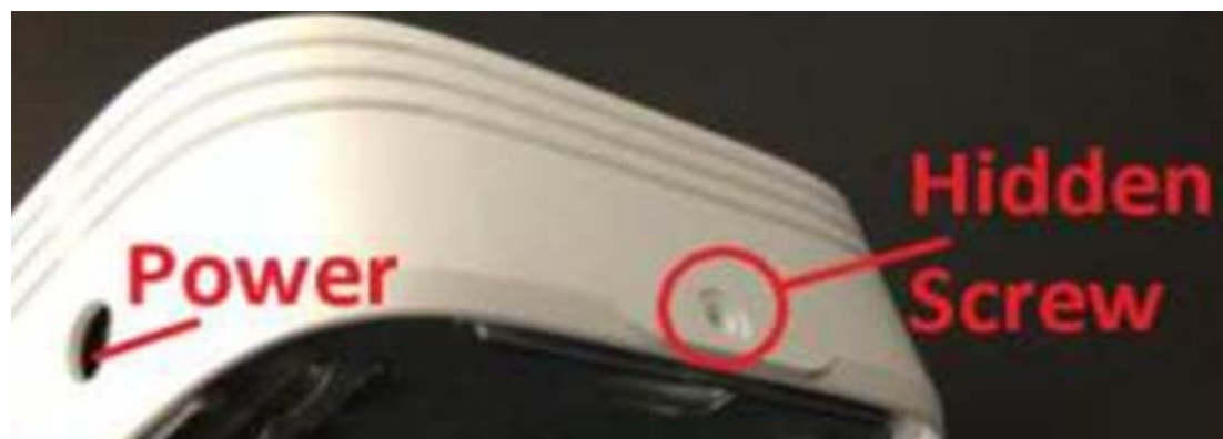
Figure 4 The AP may be secured into the bracket with a hidden tamper resistant screw
