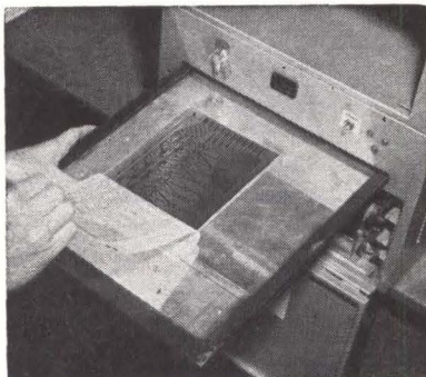
DRY IMAGE of circuit is transferred from paper to copper in processor to produce chemical resist pattern
