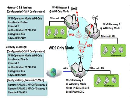
WDS (Wireless Distributed System) Only mode drives a WiFi gateway to be a bridge for its wired Intranet and a repeater to extend distance. You can use multiple WiFi gateways as a WiFi repeater chain with all gateways setup as "WDS Only" mode. All gateways can communicate with each other through WiFi. All wired client hosts within each other in the scenario. Only one gateway within repeater chain can be DHCP
