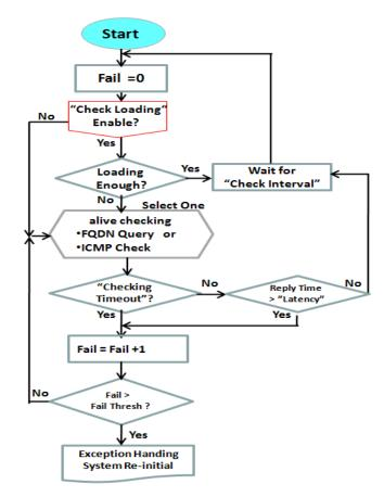
It is necessary to monitor connection status continuous. To do it, "ICMP Check" and "FQDN Query" are used to check. When there is trafiic of connection, checking packet will waste bandwidth. Response time of replied packets may also increase. To avoid "Network Monitoring" work abnormally, enabling "Checking Loading" option will stop connection check when there is traffic. It will wait for another "Check Interval" and then check loading again.
