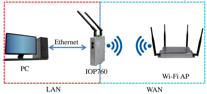
The IOP760 is configured in "**Bridge**" mode which basically means that the PC is bridged to the production network and that PC operates as if it exists directly on the production network.
