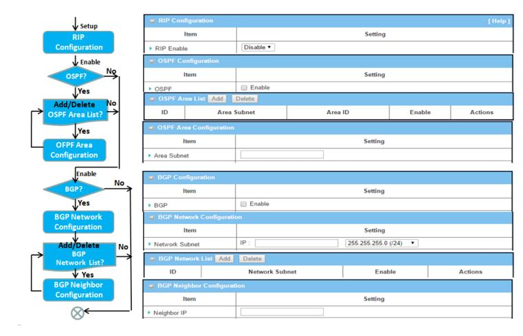
Dynamic Routing, also called adaptive routing, describes the capability of a system, through which routes are characterized by their destination, to alter the path that the route takes through the system in response to a change in network conditions.
