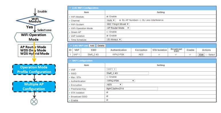
Due to optional module(s) and frequency band, you need to setup module one by one. For each module, you need to specify the operation mode, and then setup the virtual APs for wireless access.
