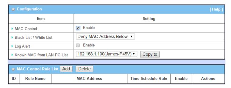
"MAC Control" function allows you to assign the accessibility to the gateway for different users based on device's MAC address. When the administrator wants to reject the traffics from some client hosts with specific MAC addresses, he can use the "MAC Control" function to reject with the black list configuration.
