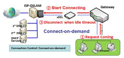
Connect-on-demand: This gateway won't start to establish Internet connection until local data is going to be sent to WAN side. After normal data transferring between LAN and WAN sides, this gateway will disconnect WAN connection if idle time reaches value of Maximum Idle Time.
