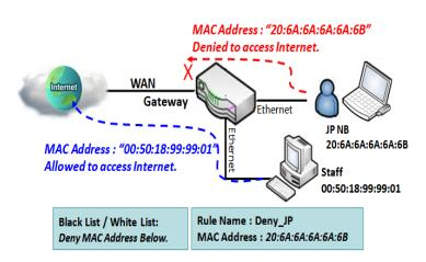
As shown in the diagram, enable the MAC control function and specify the "MAC Control Rule List" is a black list, and configure one MAC control rule for the gateway to deny the connection request from the "JP NB" with its own MAC address 20:6A:6A:6A:6A:6B.
