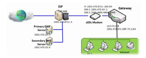
Above diagram depicts the IPv6 IP addressing, type in the information provided by your ISP to setup the IPv6 network.
