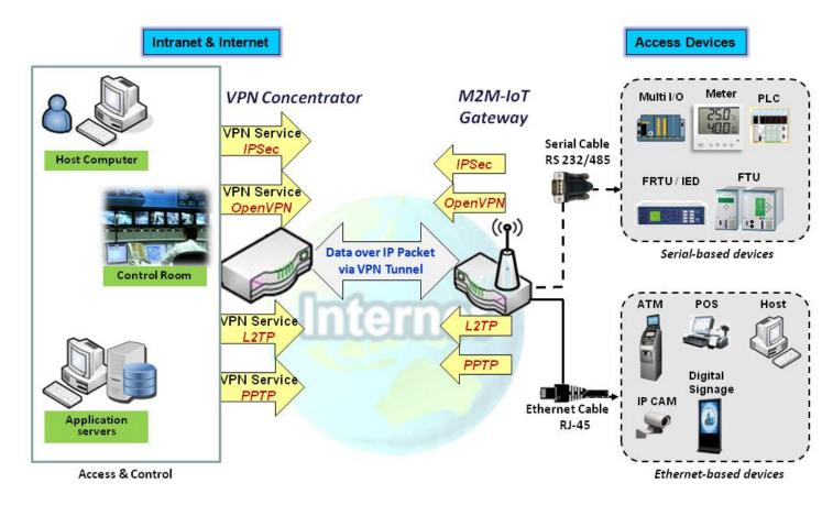
The product series supports different tunneling technologies to establish secure tunnels between multiple sites for data transferring, such as IPSec, OpenVPN, L2TP (over IPSec), PPTP and GRE. Besides, some advanced functions, like Full Tunnel, Tunnel Failover, Tunnel Load Balance, NetBIOS over IPSec, NAT Traversal and Dynamic VPN, are also supported.
