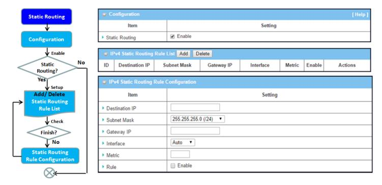
"Static Routing" function lets you define the routing paths for some dedicated hosts/servers or subnets to store in the routing table of the gateway. The gateway routes incoming packets to different peer gateways based on the routing table. You need to define the static routing information in gateway routing rule list.
