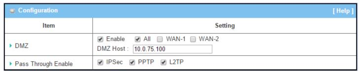
gateway firewall. Activate the feature and specify the DMZ host with a host in the Intranet when needed.
