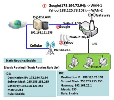
When the administrator of the gateway wants to specify what kinds of packets to be transferred via which gateway interface and which peer gateway to their destination. It can be carried out by the "Static Routing" feature. Dedicated packet flows from the Intranet will be routed to their destination via the pre-defined peer gateway and corresponding gateway interface that are defined in the system routing table by manual.
