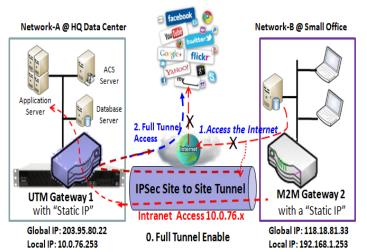
In "Site to Site" scenario, client hosts in remote site can access the enterprise resources in the Intranet of HQ gateway via an established IPSec tunnel, as described above. However, Internet access originates from remote site still go through its regular WAN connection. If you want all packets from remote site to be routed via this IPSec tunnel, including HQ server access and Internet access, you can just enable the "Full Tunnel" setting. As a result, every time users surfs
