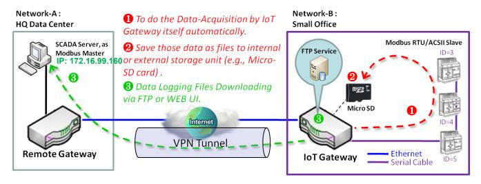
As illustrated, when the connection to a remote Modbus Master broken, the Modbus Gateway will activate the data logging proxy function and execute the pre-defined data acquisition task by itself.
