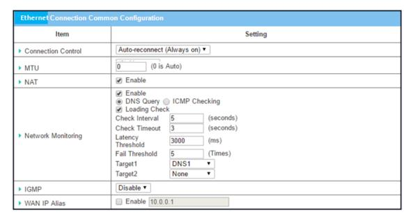
There are some important parameters to be setup no matter which WAN type is selected. You should follow up the rule to configure.
