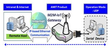
Data is Transferred between Remote Host and Serial Device Directly
