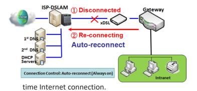
**Auto-reconnect:** This gateway will establish Internet connection automatically once it has been booted up, and try to reconnect once the connection is down. It's recommended to choose this scheme if for mission critical applications to ensure full-
