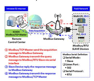
The IoT Gateway serves as a Modbus gateway to communicate with the Modbus TCP Master, the SCADA Server, located at remote control center for Modbus device accessing.
