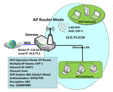
This mode allows you to get your wired and wireless devices connected to form the Intranet of the wireless gateway, and the Intranet will link to the Internet with NAT mechanism of the gateway. So, this gateway is working as a WiFi AP, but also a WiFi hotspot for Internet accessing service. It means local WiFi clients can associate to it, and go to Internet. With its NAT mechanism, all of wireless clients don't need to get public IP addresses from ISP.
