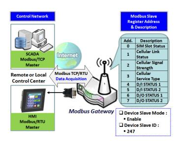
In addition to behave as a Modbus Gateway, there is an integrated Modus Slave option for providing some device status, like Cellular Network Status, device DI/DO status, to remote Modbus Master via Modbus communication.
