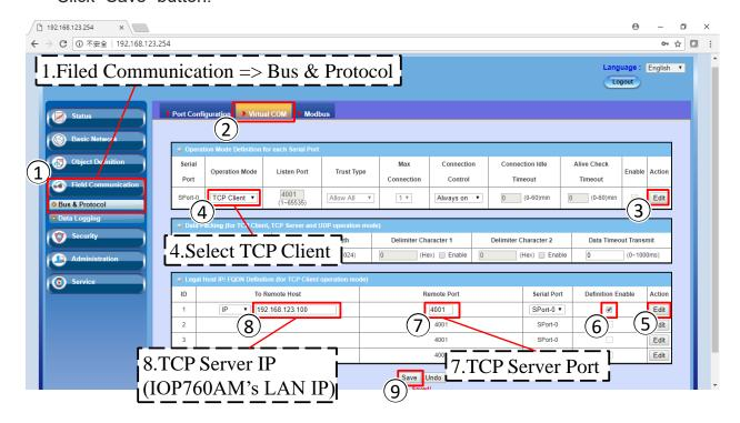
\*The IP of "Remote Host" is the IOP760's LAN IP.
