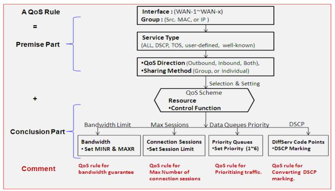
In above diagram, a QoS rule is organized by the premise part and the conclusion part. In the premise part, you must specify the WAN interface, host group, service type in the packets, packet flow direction to be watched and the sharing method of group control or individual control. However, in the conclusion part, you must make sure which kind of system resource to distribute and the control function based on the chosen system resource for the rule.
