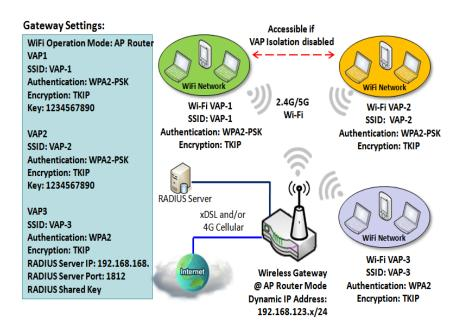
VAP (Virtual Point) is Access function to partition wireless network into multiple broadcast domains. It can simulate multiple APs in one physical AP. This wireless gateway supports up to 8 VAPs. For each VAP, you need to setup SSID, authentication and encryption to control Wi-Fi client access.
