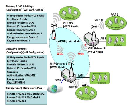
WDS hybrid mode includes both WDS and AP Router mode. WDS Hybrid mode can act as an access point for its WiFi Intranet and a WiFi bridge for its wired and WiFi Intranets at the same time. Users can thus use the features to build up a large wireless network in a large space like airports, hotels or campus.
