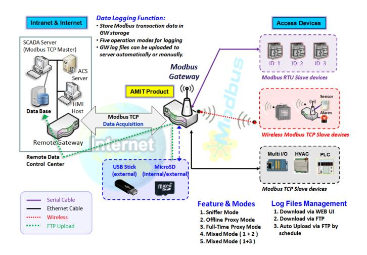
The Modbus Cellular Gateway provides a complete data logging function for collecting the Modbus transaction data for application requirements. There are some data logging schemes to meet different management requirements. They are the Sniffer Mode, Offline Proxy Mode, Full-Time Proxy Mode, and
