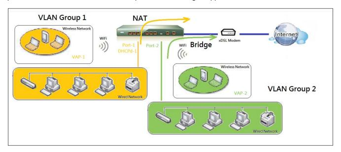
A port-based VLAN is a group of ports on an Ethernet or Virtual APs of Wired or Wireless Gateway that form a logical LAN segment. Following is an example.
