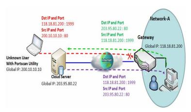
As shown in the diagram, Gateway has the IP address of 118.18.81.200 for WAN interface and 192.168.1.253 for LAN interface. It serves as a NAT gateway. Users in Network-A initiate to access cloud server through the gateway. Sometimes, unknown users will simulate the packets but use different source IP to masquerade. With the SPI feature been enabled at the gateway, it will block such packets from unknown users.
