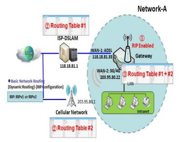
The Routing Information Protocol (RIP) is one of the oldest distance-vector routing protocols, which employs the hop count as a routing metric. RIP prevents routing loops by implementing a limit on the number of hops allowed in a path from the source to a destination. The maximum number of hops allowed for RIP is 15. This hop limit, however, also limits the size of networks that RIP can support. A hop count of 16 is considered an infinite distance, in other words the route is
