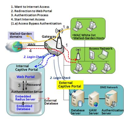
In contrast, for internal captive portal, you will only select "Internal RADIUS Server" option for user authentication. The user account database can be an embedded database, an external AD database or an external LDAP database. However, the UAM server is not necessary for this case and that the captive portal Web site is embedded in the device.
