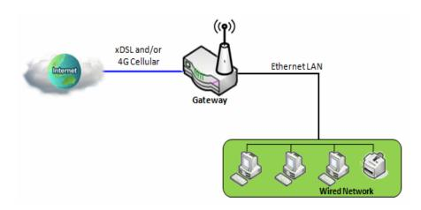
The Local Area Network (LAN) can be used to share data or files among computers attached to a network. Following diagram illustrates the network that wired and interconnects computers.
