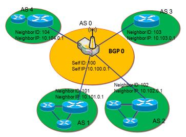
Border Gateway Protocol (BGP) is a standard exterior gateway protocol designed to exchange routing and reachability information between autonomous systems (AS) on the Internet. It usually makes routing decisions based on paths, network policies, or rule-sets.
