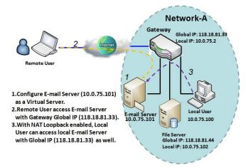
"Virtual Server" allows you to access servers with the global IP address or FQDN of the gateway as if they are servers existed in the Internet. But in fact, these servers are located in the Intranet and are physically behind the gateway. The gateway serves the service requests by port forwarding the requests to the LAN servers and transfers the replies from LAN servers to the requester on the WAN side. As shown in example, an E-mail virtual
