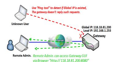
"Discard Ping from WAN" makes any host on the WAN side can't ping this gateway reply any ICMP packets. Enable the Discard Ping from WAN function to prevent security leak when local users surf the internet.
