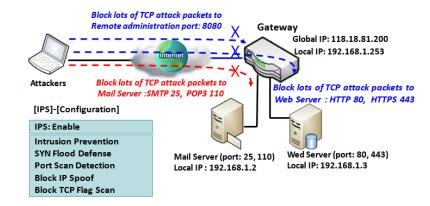
As shown in the diagram, the gateway serves as an E-mail server, Web Server and also provides TCP port 8080 for remote administration. So, remote users or unknown users can request those services from Internet. With IPS enabled, the gateway can detect incoming attack packets, including the TCP ports (25, 80, 110, 443 and 8080) with services. It will block the attack packets and let the normal access to pass through the
