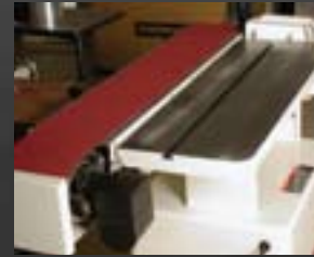
Sanding belt can be locked in at vertical, horizontal and any angle in between
