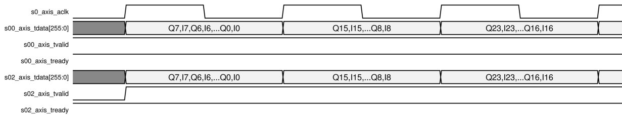
Figure 69: RF-DAC I/Q Input to I/Q Output Data Timing
