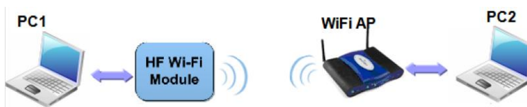
Figure 56. STA Interface Debug Connection
