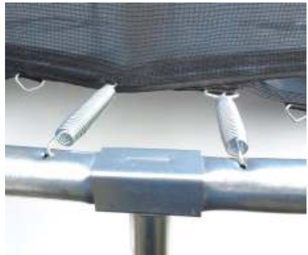
One spring attached through the enclosure netting and the other spring still attached directly to the jumping mat.
