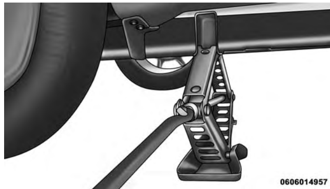
Rear Jack Engaged With Jack Handle
