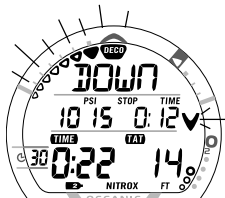
Fig. 80 - NORM DELAYED VIOLATION #1 MAIN
