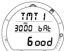
Fig. 5 - Transmitter 1 Battery Status (Good)
