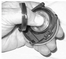
Fig. 129 - VT3 BATTERY INSTALLATION
