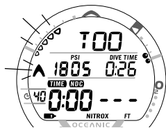
Fig. 82 - DELAYED VIOLATION #3 MAIN
