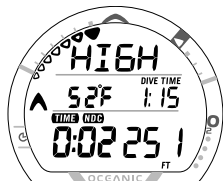
Fig. 121 - FREE DIVE MAIN (During TLBG ALARM)
