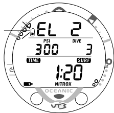
Fig. 3 - Low Battery Alarm
