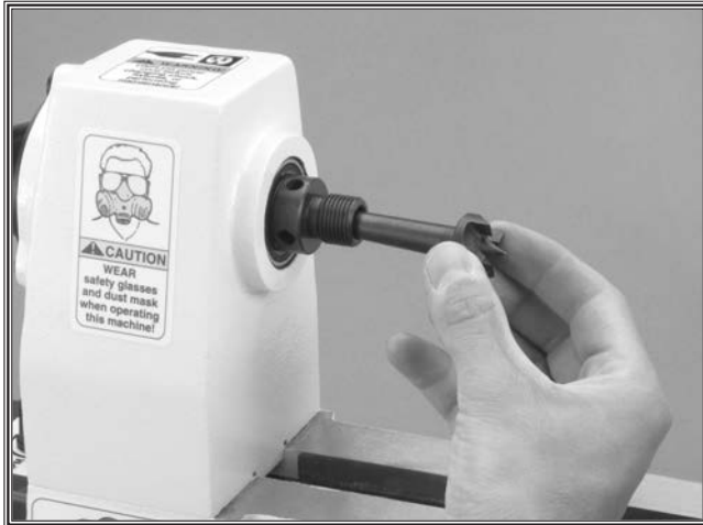
Figure 9. Installing spur center into headstock spindle.
