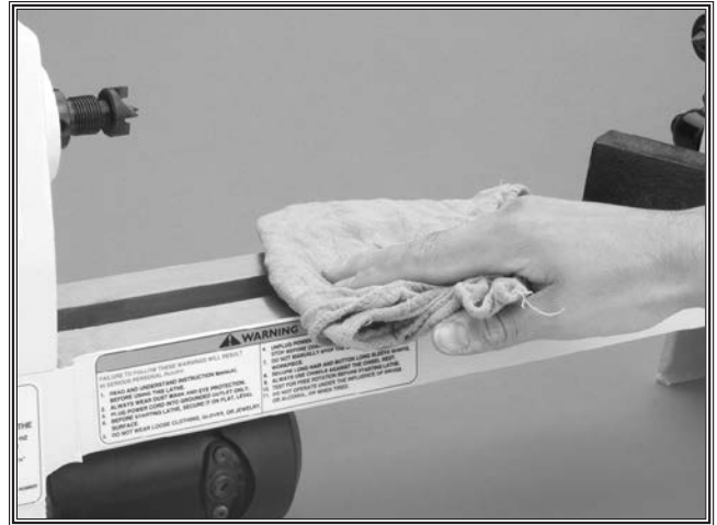
Figure 31. Cleaning/lubricating unpainted part of the bed.
