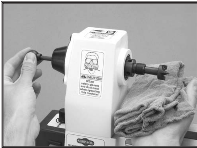
Figure 10. Removing spur center with knock-out tool.
