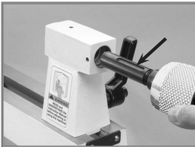
Figure 14. Tailstock barrel alignment slot.
