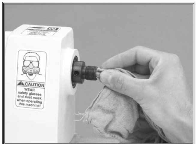
Figure 32. Cleaning spindle tapers.
