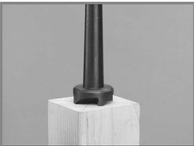
Figure 25. Spur center properly embedded into workpiece.
