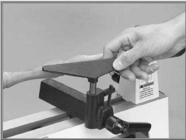
Figure 29. Removing tool rest.
