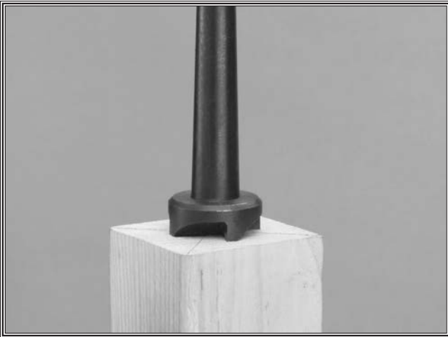
Figure 1. Center fully embedded in workpiece.
