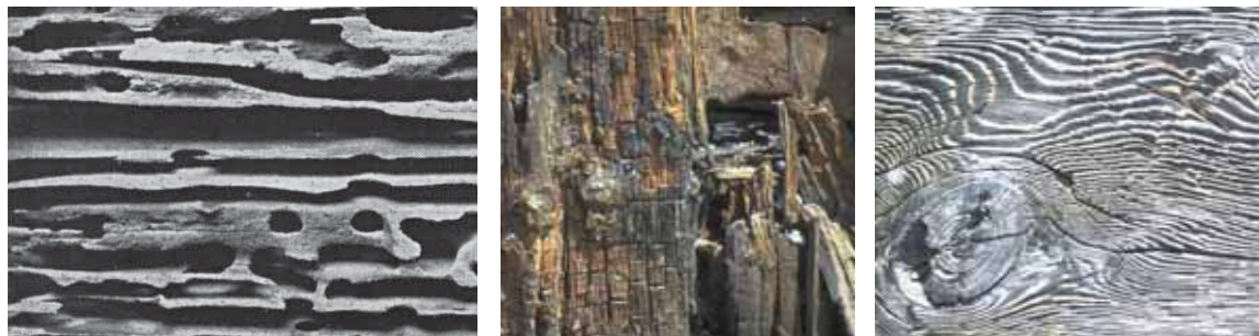
Figure 1. Wood products that are in contact with the ground or exposed to weather can be damaged by a variety of damaging insects (left), fungi (middle), and marine borers, as well as by the weather itself (right).
