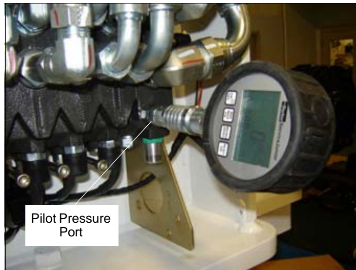
Figure 3— Gauge On Pilot Pressure Quick Disconnect
