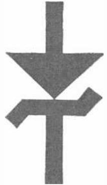
In essence, a zener diode is a device which, when saturated in the reverse direction, will maintain an almost constant voltage across its terminals. The most popular application for a device of this type is, of course, voltage regulation.
