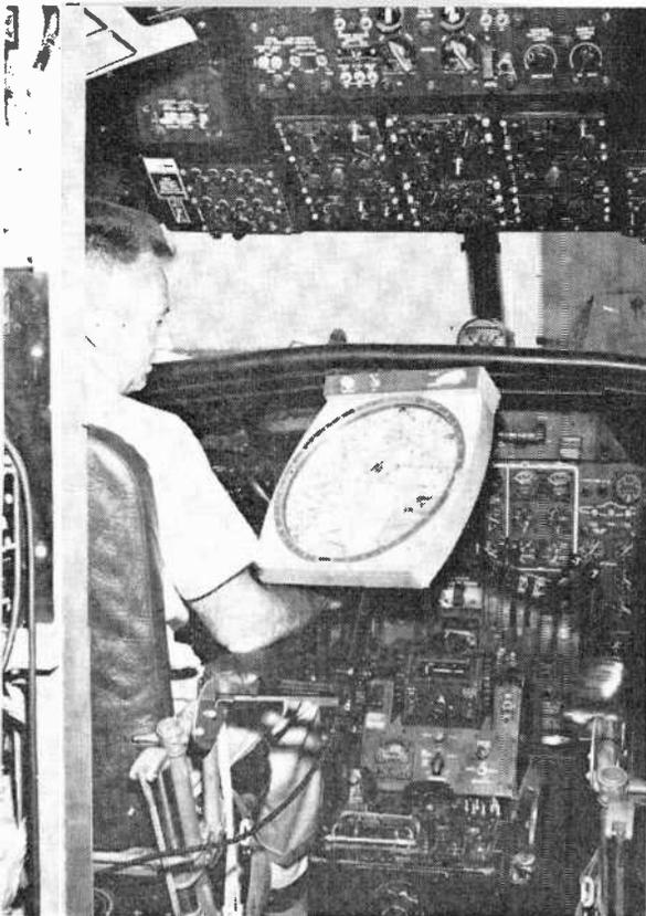
Automatic flight course display developed by IT&T enables pilot to navigate by looking at map (left) showing his course and position. With IT&T display, pilot can easily guide his plane along any course he wishes.
