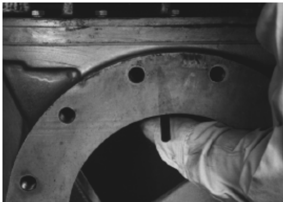
FIGURE 7-19 – DISCHARGE END CLEARANCE CHECK
