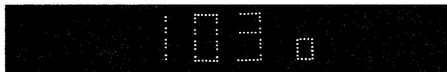
Fig. 9: A typical service mode display. The left-hand digit is the service mode number, indicating the operation being checked. The next two digits (03 here) indicate the circuit condition and/or the position of the mechanism.
