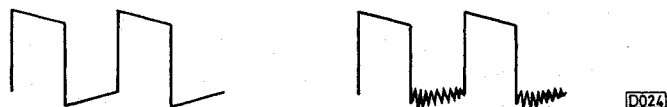
Fig. 1: Correct (left) and the incorrect waveform (right) found at pin 36 of IC106 in the Ferguson 3V65.
