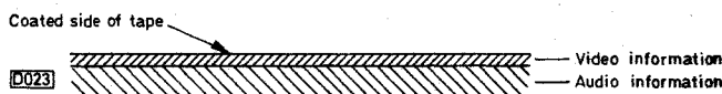
Fig. 3: The audio signals are recorded at a deeper level in the tape's oxide coating than the video signals.
