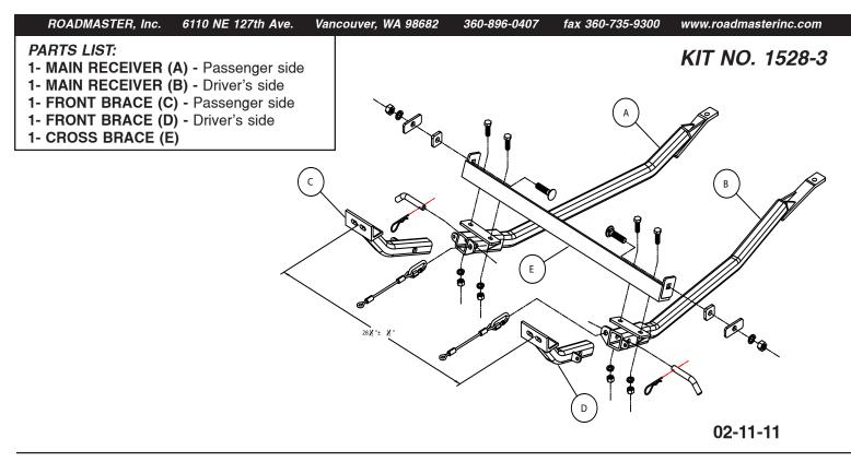
**IMPORTANT:** All baseplates **must** be assembled with all the bolts left loose for final adjustment and positioning (before tightening) unless otherwise instructed. All bolts **must** be torqued for proper strength. If more than one bolt is used per fastening point, the diagram may only show one.
