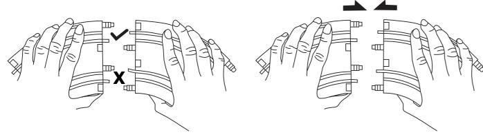
Adjust the distorted joints before joining tracks. Do not join the tracks together if the joints are distorted.
