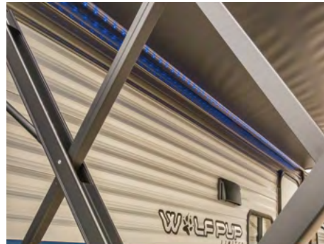
Exterior LED Light Strip at Awning
