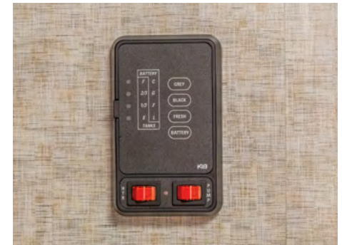
Monitor Panel for Tanks and Battery Level
