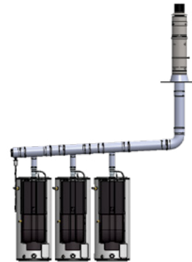
ROOM AIR COMMON VENT CONFIGURATION VERTICAL EXHAUST DEMAND DUO®
