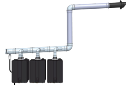
ROOM AIR WITH HORIZONTAL EXHAUST (NEW)
