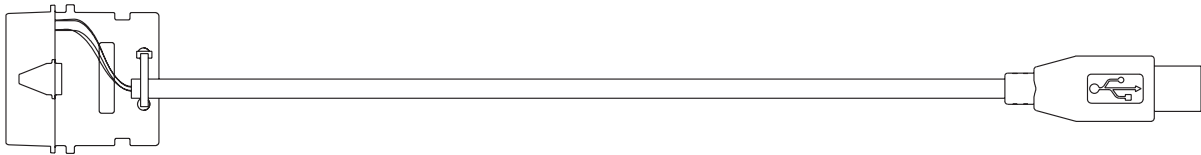
Figure 3-2 Mobile & Repeater Rear Programming Cable PMKN4010_
