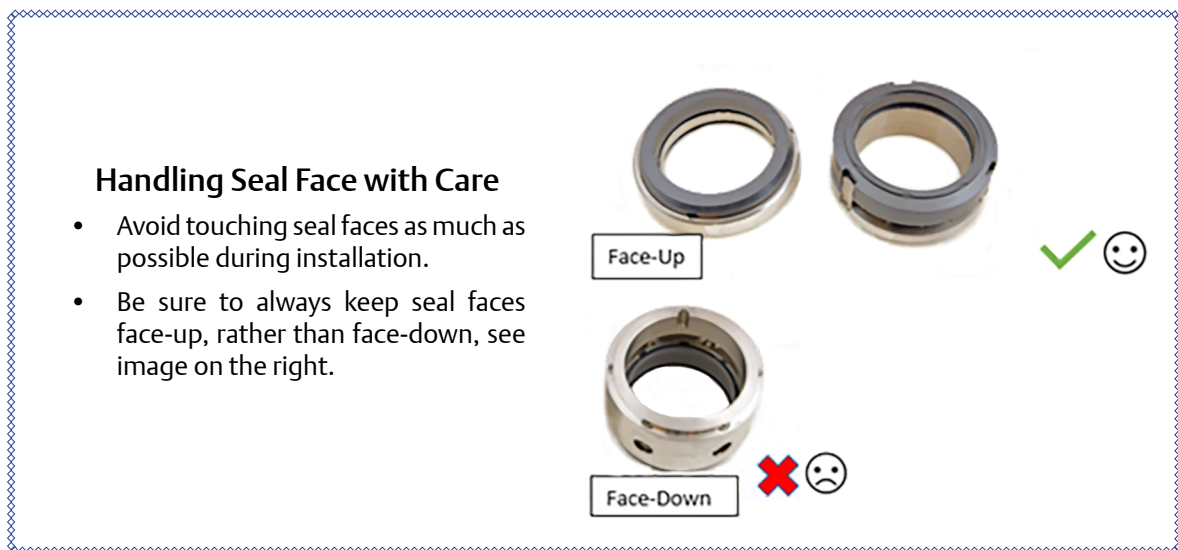
Figure 5-40. Handling Seal Face with Care
