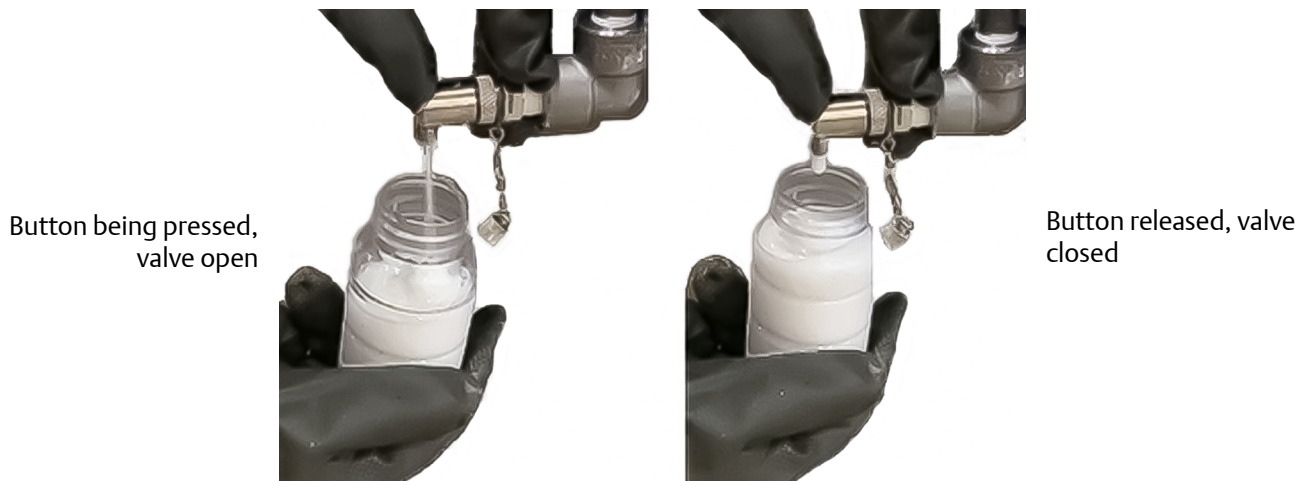
Figure 5-5. Operating the Oil Sampling Valve
