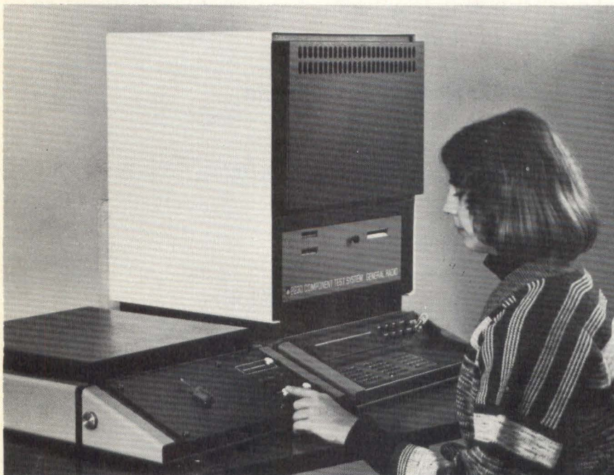
When they discovered that software development costs for their Model 2230 circuit testing system were soaring and that development efforts were duplicating a current development system, engineers at GenRad's Test Systems Div. replaced the unit's in-house designed microcomputer (built around a National Semiconductor IMP-16 CPU) with a fully documented Digital Equipment Corp. LSI-11.
