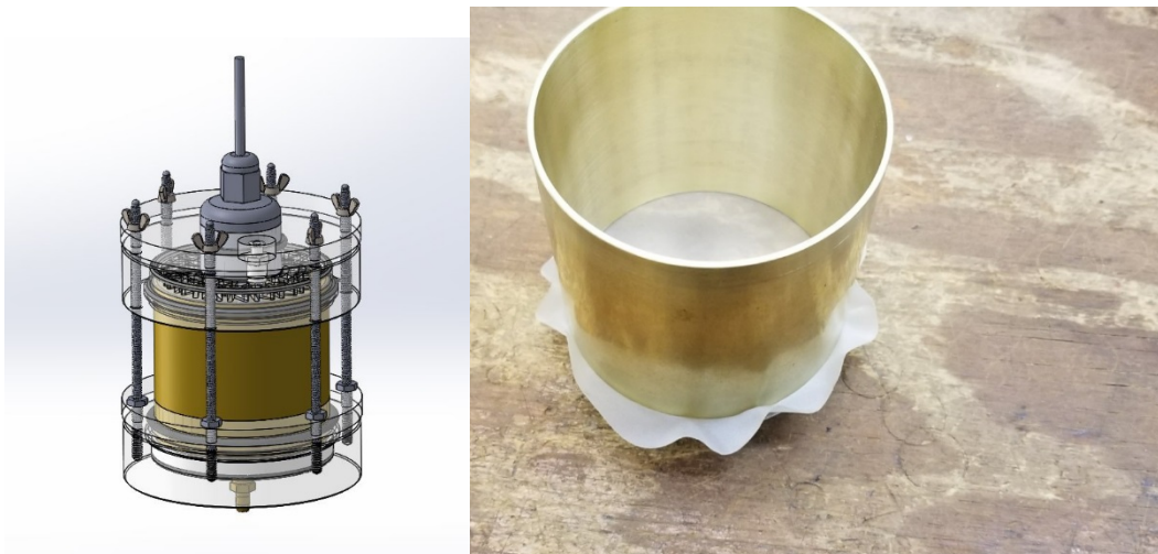
Figure 1.4. The Tempe Cell for custom calibrations, soil water retention curves
