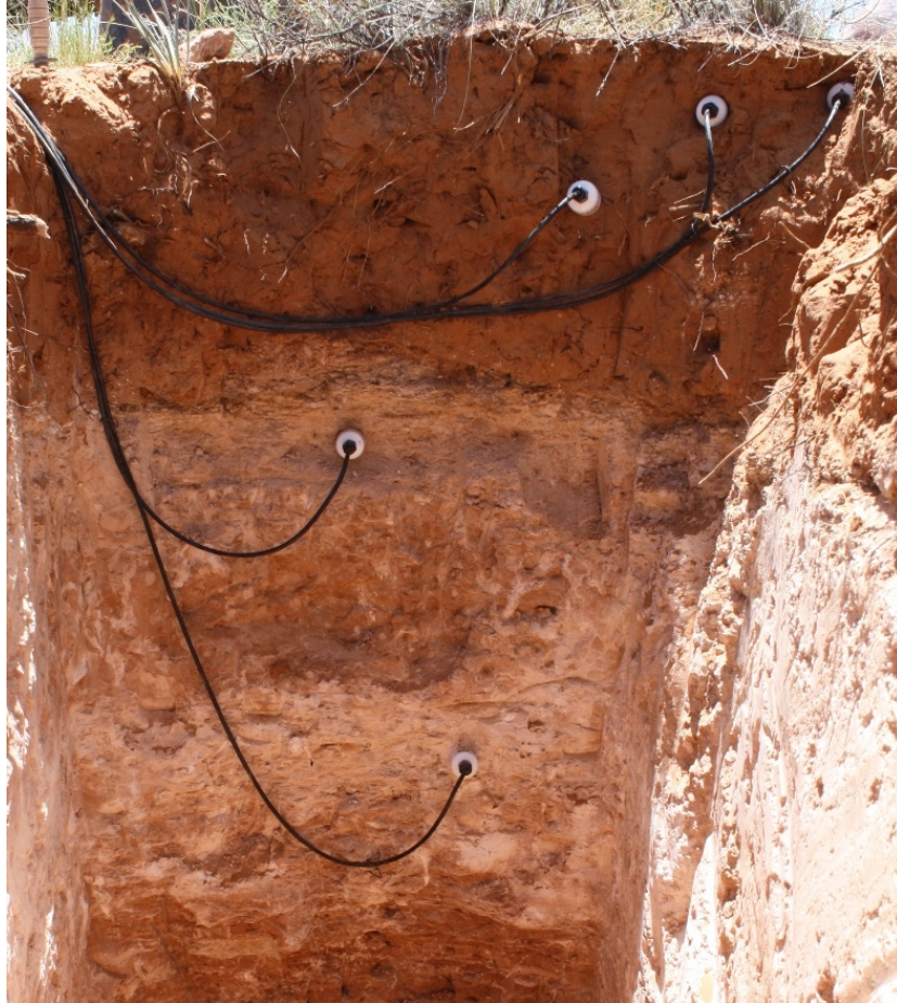
HydraProbe installation at a typical USDA NRCS SNOTEL Site. Picture compliments of USDA NRCS in Salt Lake City, Utah.
