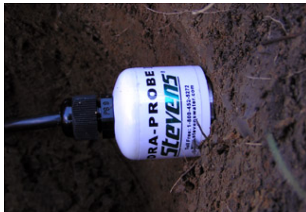
Figure 2.6 HydraProbe Installed in undisturbed soil.
