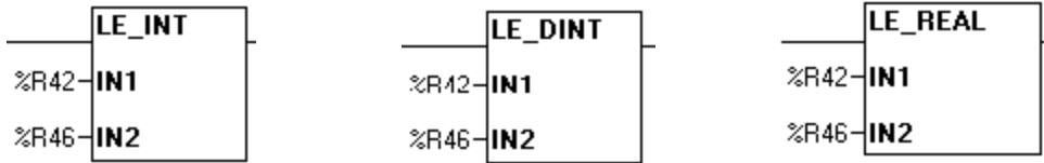
LESS THAN OR EQUAL DINT LESS THAN EQUAL1 REAL LESS THAN EQUAL
