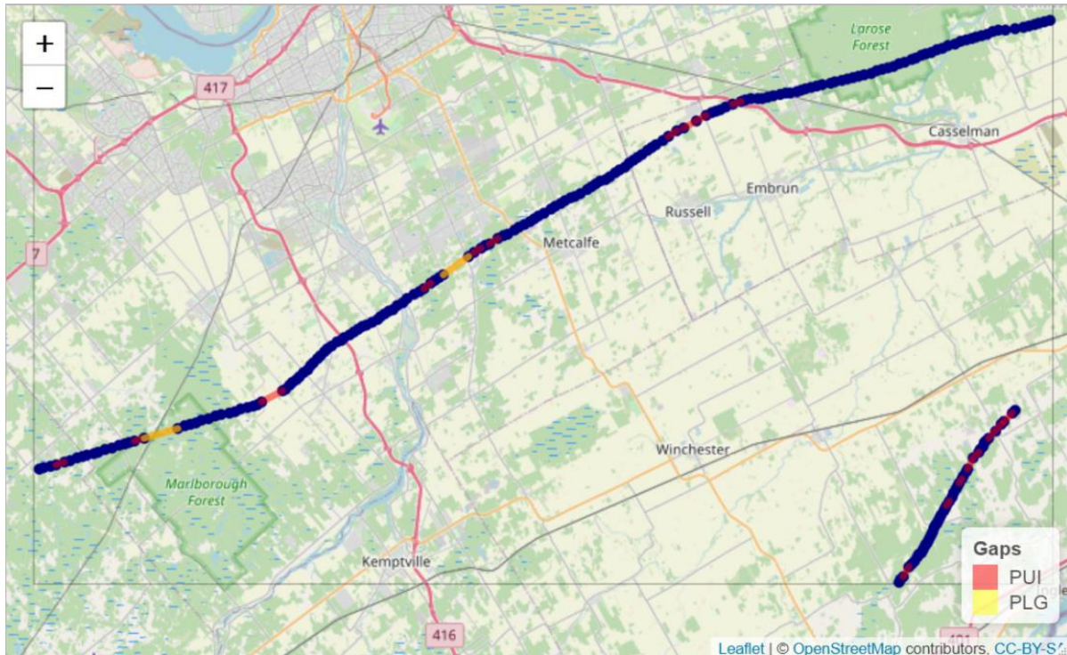
Figure 2: Throttled operations for target C0654A September 2020. Red portions are a failure of PUI of 8 seconds, yellow are failures of PLG n=3
