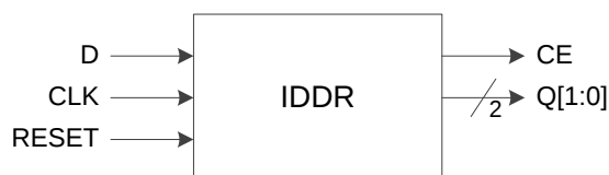
Figure 3-13 I/O Logic in DDR Input Mode
