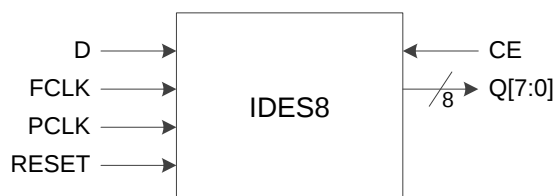
Figure 3-19 I/O Logic in IDES8 Mode
