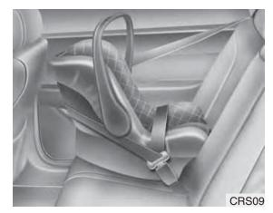
A rear-facing child seat provides restraint with the seating surface against the back of the child. The harness system holds the child in place, and in an accident, acts to keep the child positioned in the seat and reduce the stress to the fragile neck and spinal cord.
