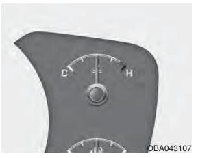
Engine coolant temperature gauge (if equipped)
