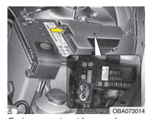
Engine compartment fuse panel Inside the fuse/relay panel covers, you can find the fuse/relay label describing
