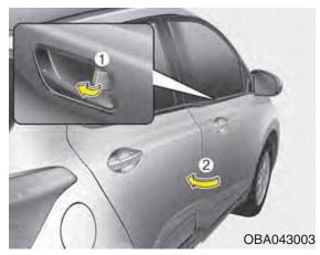
To lock a door without the key, push the inside door lock button (1) to the "Lock" position and close the door (2). (if not equipped with central door lock system)
