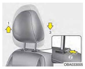
Adjusting the height up and down (if equipped)
