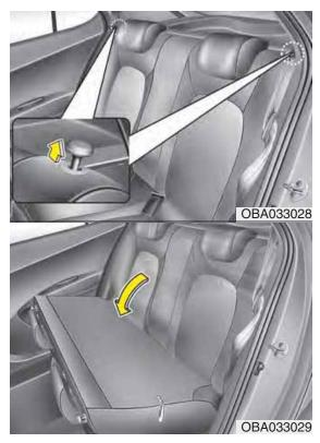
4. Pull up both sides of the seatback lever and fold the seatback toward the front of the vehicle.
