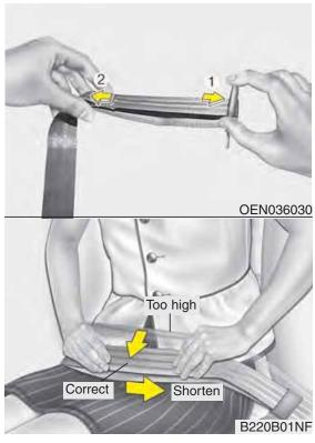
With a 2-point static type seat belt, the length must be adjusted manually so it fits snugly around your hip. Fasten the belt and pull on the loose end to tighten the belt. The belt should be placed as low as possible on your hips, not on your waist. If the belt is too high, it could increase the possibility of injury in an accident.
