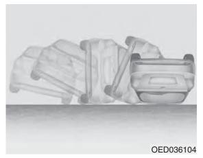
Air bags may not inflate in rollover accidents because air bag deployment could not provide protection to the occupants. However, side impact and curtain air bags may inflate when the vehicle is rolled over by a side impact collision, if the vehicle is equipped with side impact air bags and curtain air bags
