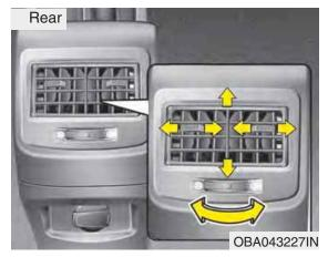
The outlet vents can be opened or closed separately using the thumbwheel.
