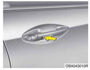
Carrying the smart key, you may lock and unlock the vehicle doors and tailgate/trunk.
