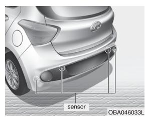
The Rear Parking Assist System aids the driver during backward movement of the vehicle by chiming if any object is sensed within the distance of about 120 cm (47 in) behind the vehicle. This is a supplemental system that senses objects within the range and location of the sensors, it can not detect objects in other areas where sensors are not installed.
