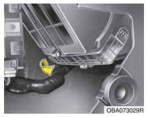
Remove the climate control air filter cover.
