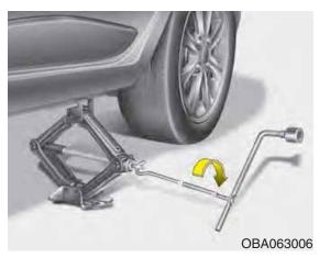
8. Insert the jack handle into the jack and turn it clockwise, raising the vehicle until the tire clears the ground. Make sure the vehicle is stable on the jack.
