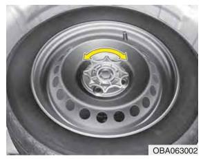
Removing and storing the spare tire Turn the tire hold-down wing bolt counterclockwise.
