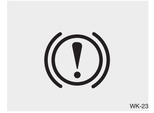
Check the Parking Brake Warning Light by placing the ignition switch to the ON position (do not start the engine).
