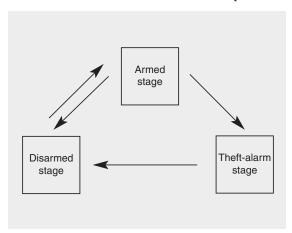
This system is designed to provide protection from unauthorized entry into the car. This system is operated in three stages: the first is the "Armed" stage, the second is the "Theft-alarm" stage, and the third is the "Disarmed" stage. If triggered, the system provides an audible alarm with the hazard warning light blinking.
