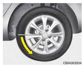
6. Loosen the wheel lug nuts counterclockwise one turn each in the order shown above, but do not remove any lug nuts until the tire has been raised off of the ground.
