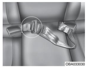
When using the rear center seat belt, the buckle with the "CENTER" mark must be used. (if equipped)
