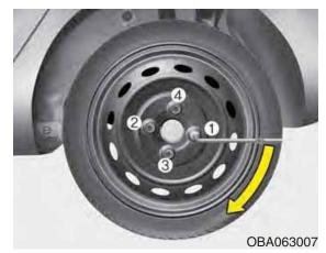
13. Use the wheel lug nut wrench to tighten the lug nuts in the order shown. Double-check each lug nut until they are tight. After changing tires, we recommend that an authorized HYUNDAI dealer tighten the lug nuts to their proper torque as soon as possible. The wheel lug nut should be tightened to 11~13 kg.m (65~79 lb.ft).
