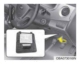
Instrument panel fuse panel Inside the fuse/relay panel covers, you can find the fuse/relay label describing the \fuse/relay name and capacity.
