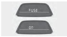
This warning light illuminates if the fuse switch in the fuse box is OFF.
