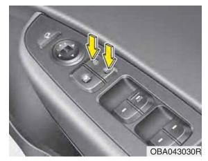
With central door lock switch (if equipped)
