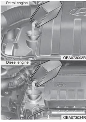
6. If it is near or at L, add enough oil to bring the level to F. **Do not overfill.**
