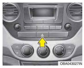
The hazard warning flasher should be used whenever you find it necessary to stop the vehicle in a hazardous location. When you must make such an emergency stop, always pull off the road as far as possible.
