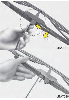
2. Press the clip (1) and slide the blade assembly downward (2).
