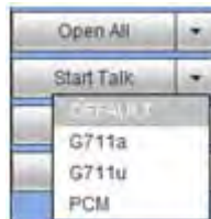
Figure 2-3 Enabling Bi-Directional Communication
