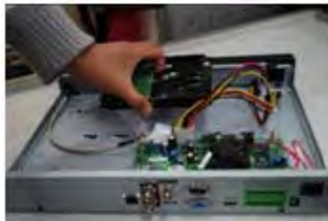
Figure 2-8 Placing the HDD
