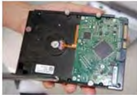
Figure 2-7 Loosening the Four Screws in the HDD Housing
