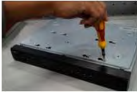
Figure 2-9 Securing the HDD to the NVR Housing
