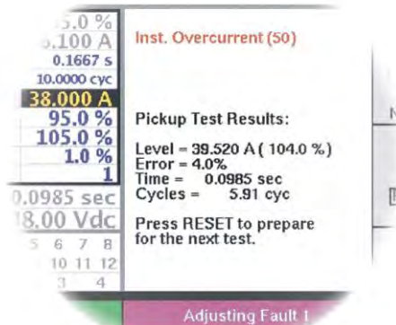
Figure 3.19 FROZEN OVERCURRENT TEST RESULTS
