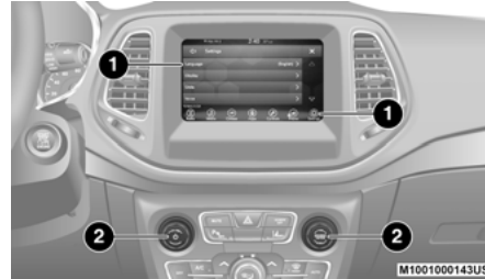
Uconnect 4 With 7-inch Display Buttons On The Touchscreen And Buttons On The Faceplate
