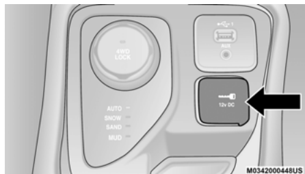
Front Power Outlet
