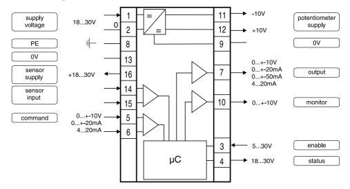
Parker electronic modules PID00A-40\* for rail mounting are compact, easy to install and provide time-saving wiring by disconnectable terminals. The digital design of the circuit results in good accuracy and optimal adaption for closed loop controls by a comfortable interface program.
