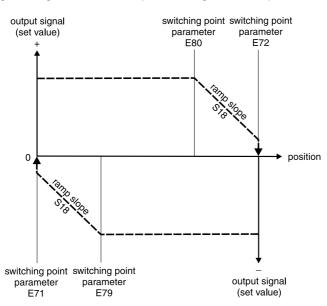
The ranges may be used independently from each other. One range is inactive, if it contains the default values given from the operating software.
