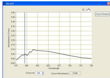
Detector saturation- Bradford measurement
