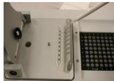
Loading samples on position A when operating within the Single Sample Mode.
