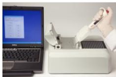
Optimal position for right handed pipetting onto the pedestals
