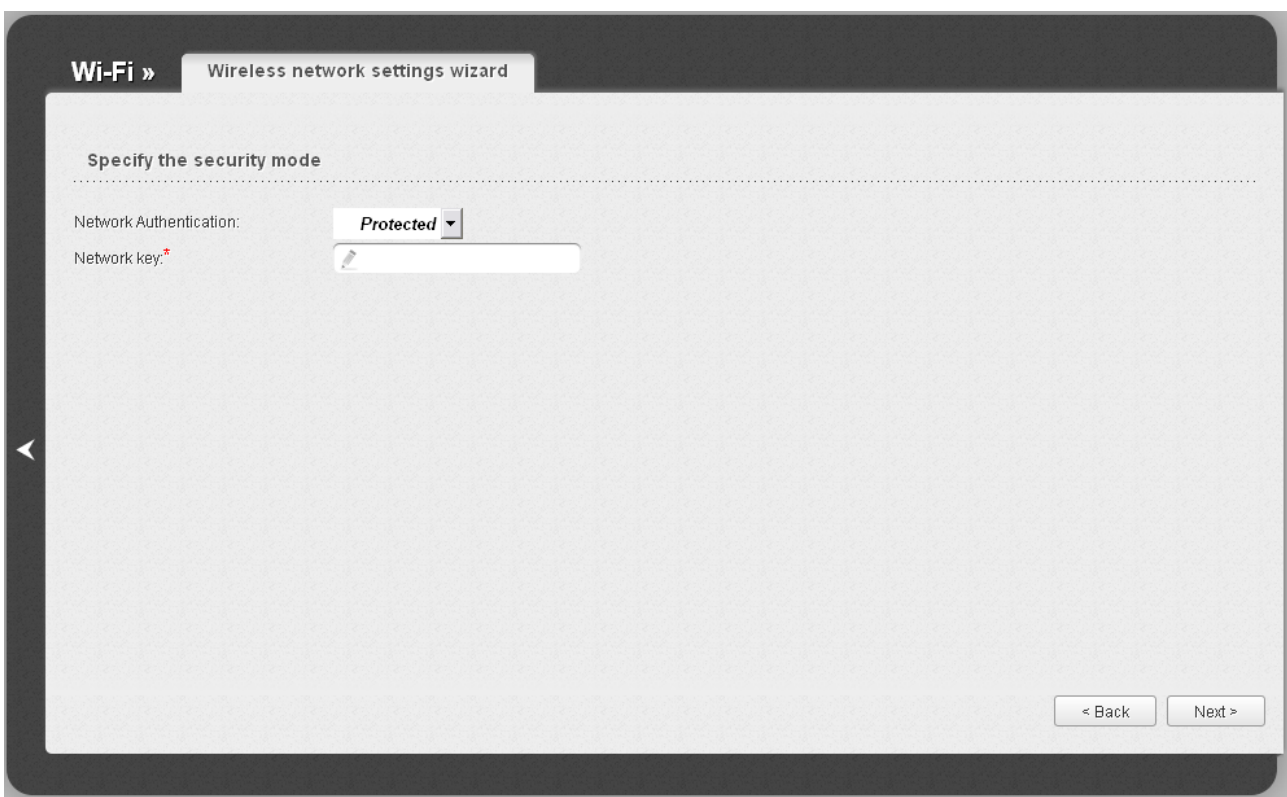
Figure 102. Page for selecting a security mode for the wireless network.
