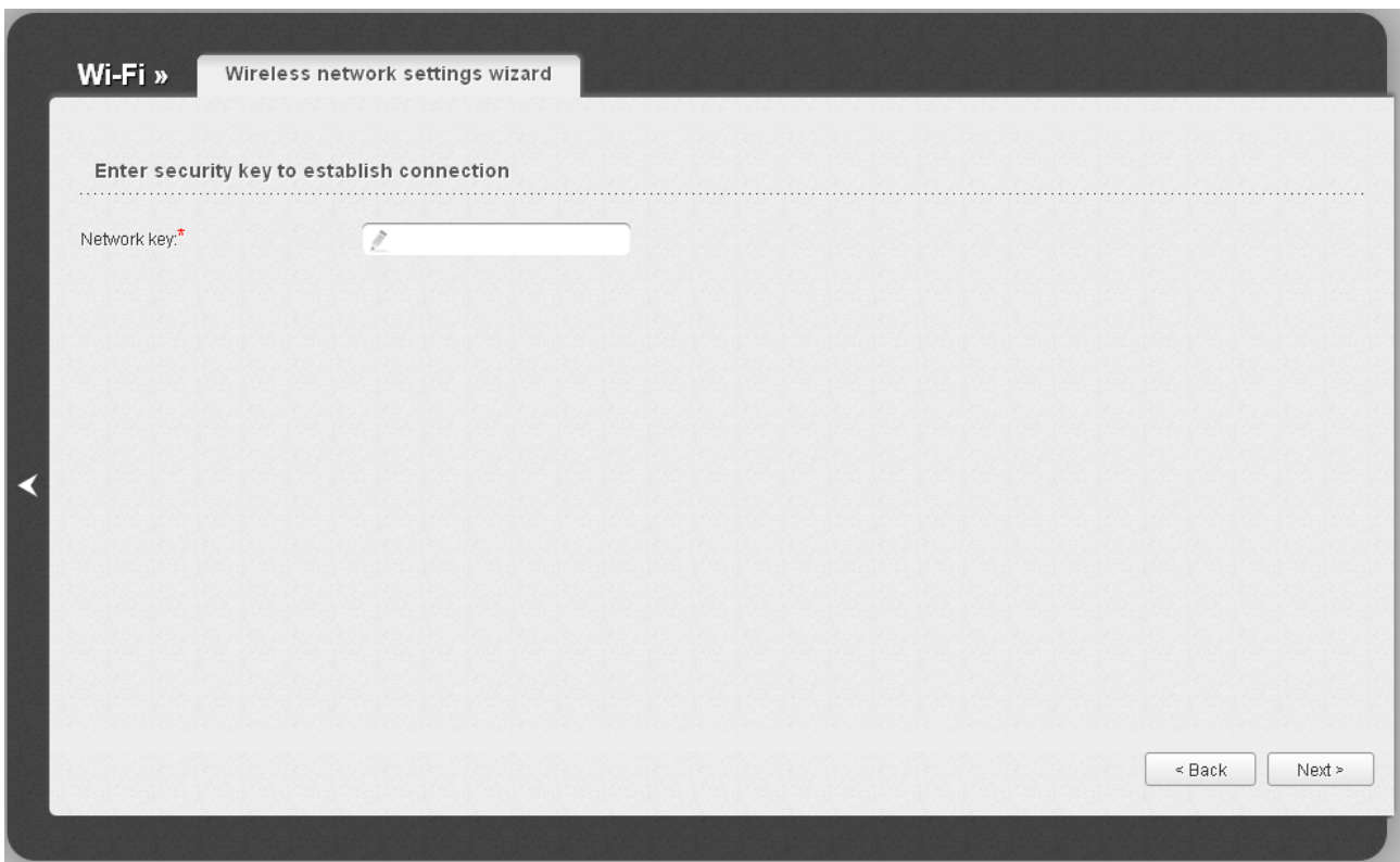
Figure 104. The page for entering the password for connection to the wireless network.
