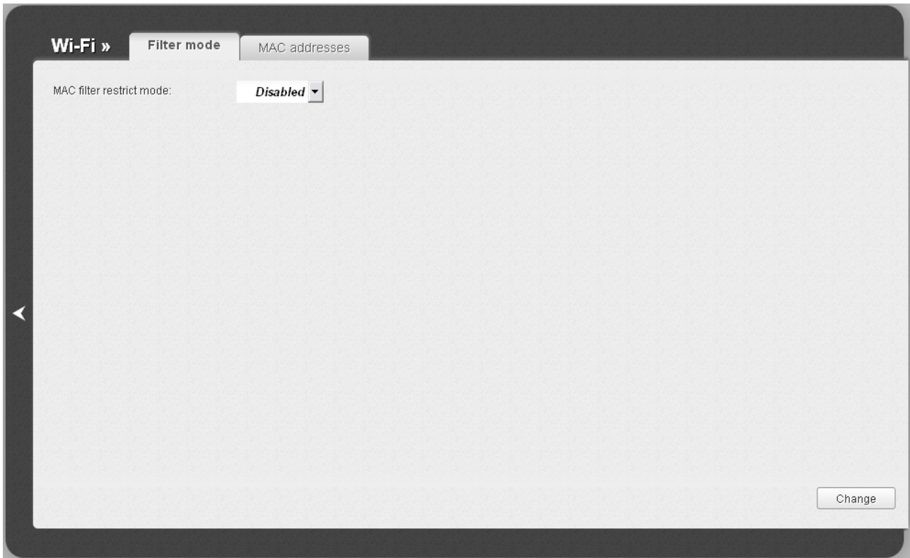
Figure 138. The MAC filter for the wireless network.
