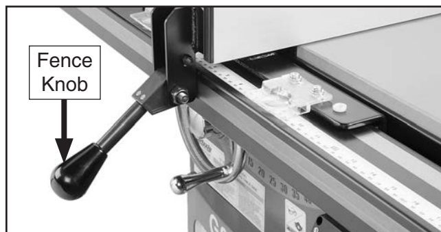
Figure 19. Fence knob installed.
