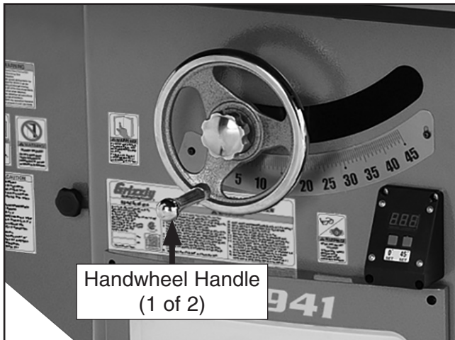
Figure 7. Handwheel handles installed on handwheels.
