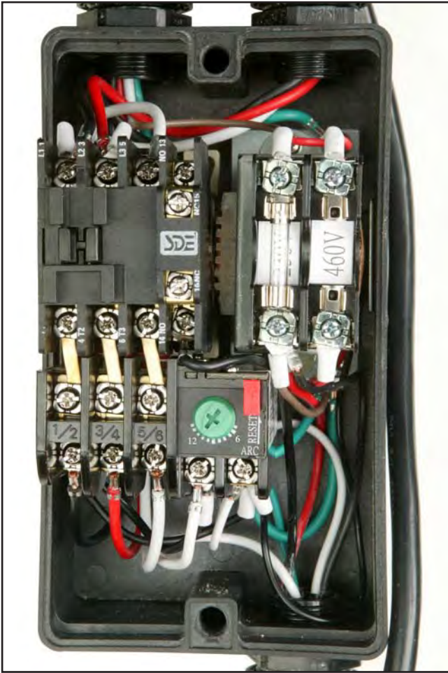
Figure 152. G0652 magnetic switch prewired to 220V, 3-phase.
