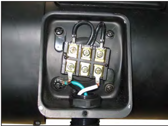
Figure 147. G0651 motor junction box.
