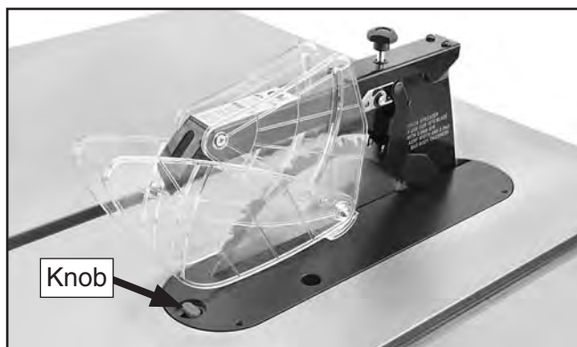
Figure 50. Blade guard and insert installed.
